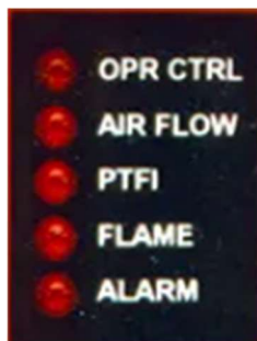
Figure 8: Relais de surveillance de flamme (FIREYE)
